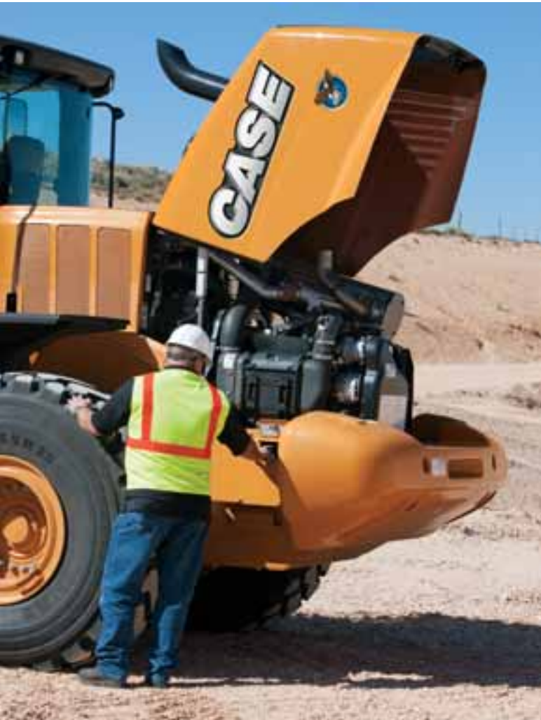
The layout of the components under the hood is optimised and results in easier maintenance.
